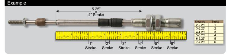
Measure from end of the support tube to the first thread on the bulk head or edge of groove. The stroke will be approximately 1.25" shorter than what you measure.
