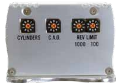
TYPICAL MULTI-SPARK CD SYSTEM ABOVE 3000 RPM
