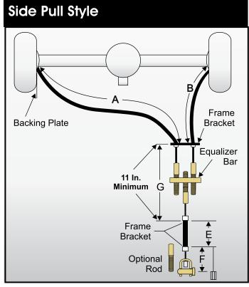
Passenger side backing plate or caliper bracket to front housing bracket.
