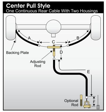
A \_\_\_\_\_\_ Passenger side backing plate or caliper bracket to front housing bracket.
